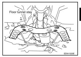
4. Loosen the center bearing mounting bracket (lower) fixing nuts with power tool.
