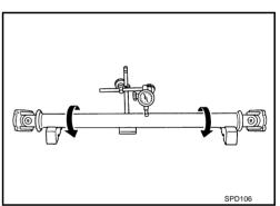
2. As shown in the figure, while fixing yoke on one side, check axial play of joint. If outside the standard, replace propeller shaft assembly.
