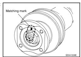
Hold the center flange using a flange wrench, and remove the lock nut.
