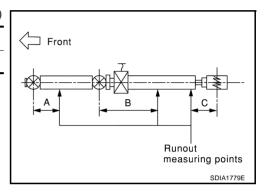
2. If the play exceeds specifications, replace propeller shaft assembly.
