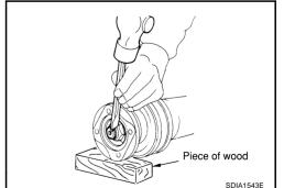
Temporality tighten the lock nut to the following torque. Loosen the lock nut, then retighten it to specified torque. For 3F80A-1VL107 (VK45DE/AWD) type, tighten the lock nut to specified torque.
